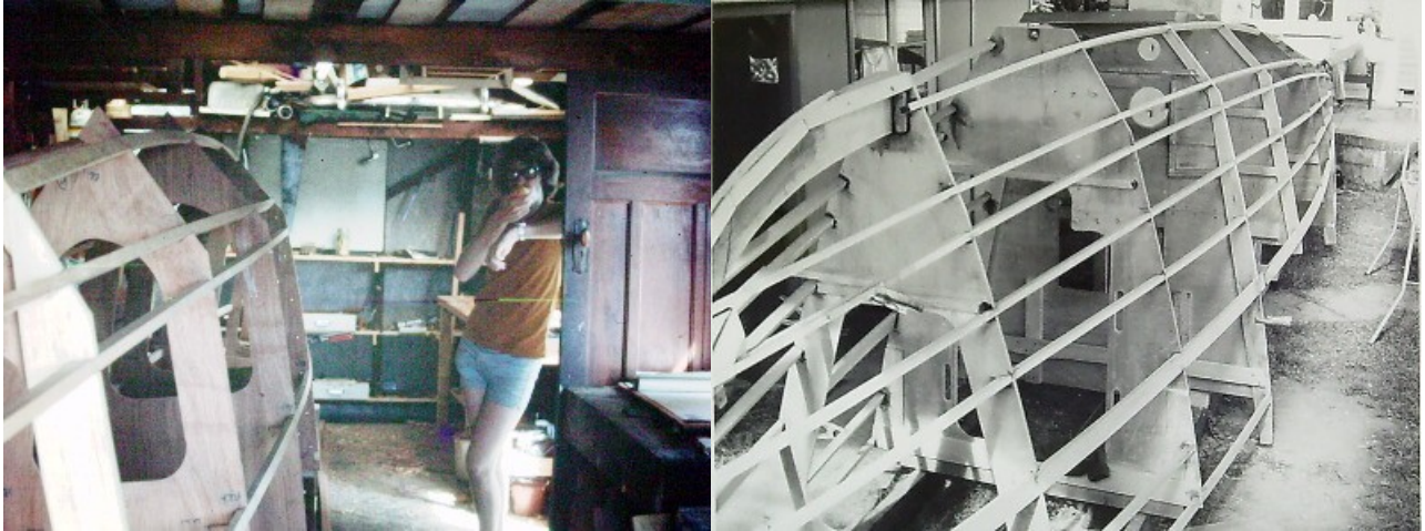
Float frames in the garage. Main hull frames in the shelter.
