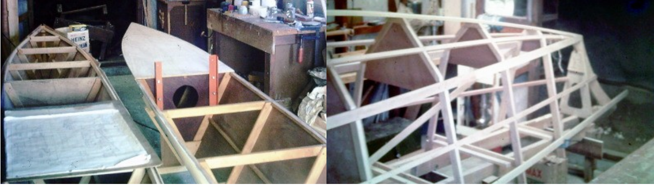
Tatu's floats and main hull were built in the garage.
