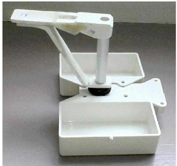
15. The second battery box was added in case the club required ballast to be added to get the boat up to the same weight as ABS models. By placing ballast in this location, it offsets the biased weight of the 4 x AA batteries.
