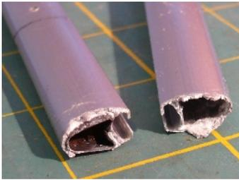
The result was a typical Seawind mast break. Right at the bottom of the bronze jointer, just where moisture will accumulate, the
