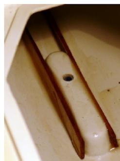
I made some fine wooden splints to lie alongside the keel box and reach forward to support the hull skin forward of the keel. These were epoxied in place and the glue smeared over the wood to seal it.
