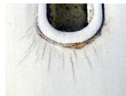
The rebuild boat does have some small cracks radiating out but not enough to cause problems yet. It will be useful to ensure that these don't get worse.
