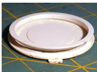
The rear hatch had split. The gluing surface is very narrow and 'Superglue' can become brittle. This joint can split without any outward indication
