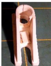
The mast support, part C3, is inadequate for the job being too short, badly designed and lacking strength. This had broken completely.
