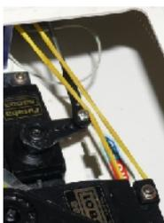
If there is a steering rod on the port side it may catch the sheet on the joint. This can be avoided by having a rubber band between the sail servo attachment post and the rear support post.
