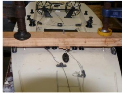
With the keel nut loosened a beam was placed across it and clamps were positioned each side.
