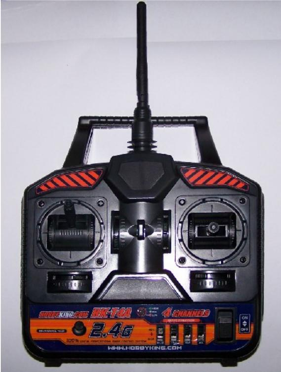
The HobbyKing system includes the HK-T4A Mode 2 4 channel transmitter and a matching HK-TR6A 6 channel receiver. These use the 2.4GHz spectrum and will seek out an unused frequency allowing many devices to be used without worrying about crystals or clashing with others.
