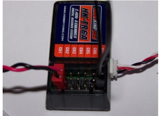
A binding plug is provided which is placed on the receiver's battery connector, the battery can be connected to any other socket. The 'Bind' button is held down while the transmitter is switched on and held for a few seconds. The receivers will flash and should show a steady light. It is important that both receivers be bound otherwise the servos may become confused by two different signal so check that both receiver's LEDs go steady.
