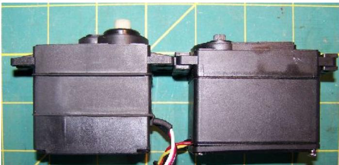
Generally it is the correct size for a sail servo though it is slightly taller above the mounting reference. The splined output shaft is considerably larger than the usual units and there is no sail arm supplied. Two output crossarms are supplied, one is a cross the other a circle. It is easy to make a simple arm from perspex or similar that can attach to the underside of one of the supplied crossarms to use as the sail arm.
