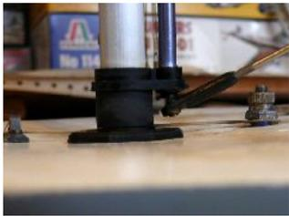
Now I had noticed that the replacement part that I had made had also broken. This was indicated by the dishing inwards of the deck and the gap between the keel nut and the deck.
