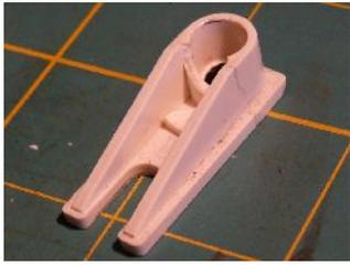
The standard part is poorly designed because the two side webs take the force to the sides of the support tube and this puts all the strain across the front of the round socket. It is also inadequate in size, both because it fails to reach under the mast step and because it is too short on the tube leading to excessive loads.
