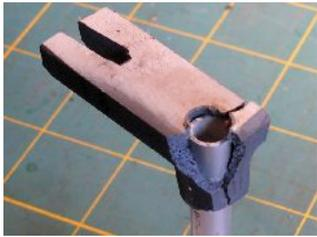
The replacement C3 part had also collapsed and there was some breaking of the deck around the keel bolt.
