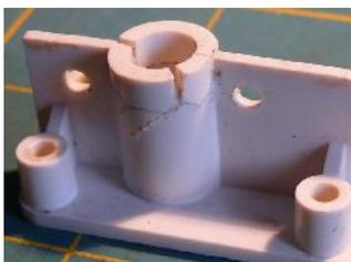
The radio support bracket that hangs off the keel tube is also breaking up, probably due to sideways movement of the keel bolt and tube.
