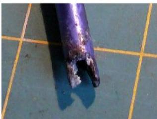
Some time ago the keel bolt tube had sheared away at the threads where it screws into the keel box. The bolt itself could support the tube but this break could leak badly as the tube is supposed to be watertight
