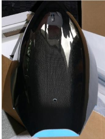
The hull is surprisingly light, it is said to be 200gram less than the ABS moulding but I didn't have a bare hull available to compare with.
