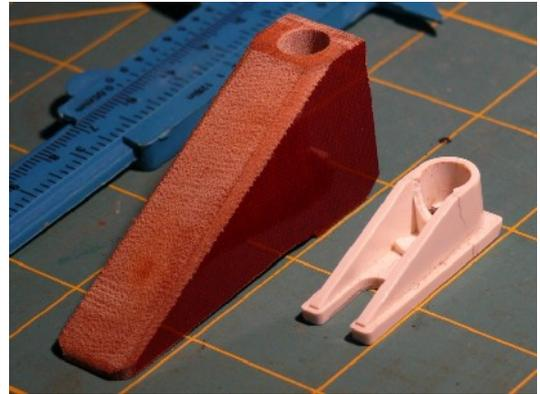
also inadequate in length and depth, it only reaches the back of the mast step and is far too shallow for adequate support.
