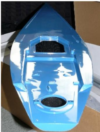
All the required mounting holes in the deck are drilled but they have no sockets to take the screws. On an ABS hull the screw holes are backed by moulded protrusions that are 'blind', if the fittings are left off the mounting holes won't leak. On this deck all the holes are drilled and will need blanking if the winches aren't fitted, or are lost.
