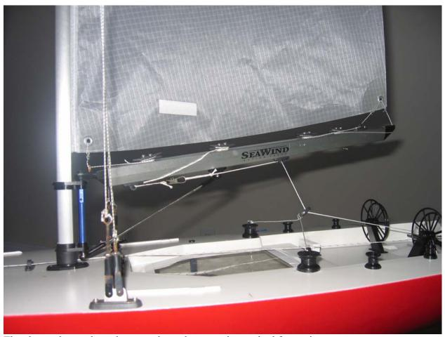
The above photos show the second attachment point method for setting camber at the base of the sail. A second line is run from the clew through a second attachment added to the top of the boom and run to an added cleat. Note that all cleats are on top of the boom to avoid catching on the shrouds of other boats.
