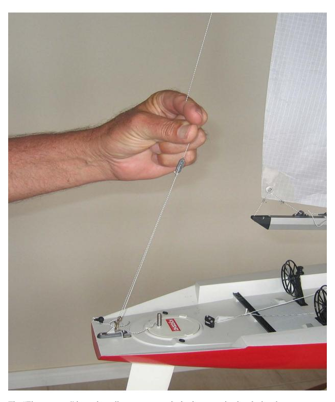
The "Fingerometer" is used to adjust or measure the backstay tension by placing the stay between the thumb and index finger and twisting.
