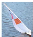
Neil Purcell had the jib boom tiedown fail in race 6 and the mast jumped out of the step but it could sail to the path for recovery (left).
