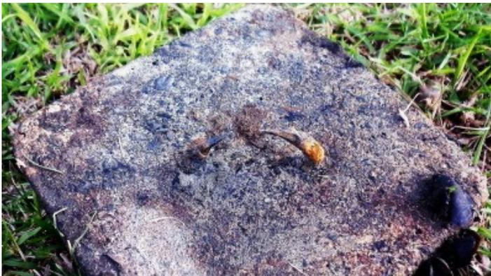
Some of the buoys were still the old design using an iron staple set in the concrete. These rust and wear and eventually break so some weights were lost when the buoy was lifted.
