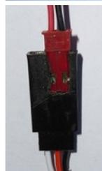
Mike has obtained a number of 120mm extension cables for servos. These can also be used to connect the battery to the receiver instead of the supplied cable that has a switch. The battery connector has a ridge on one side so that it can only be connected one way. This requires that a slot is cut in the socket end of the cable as shown.
