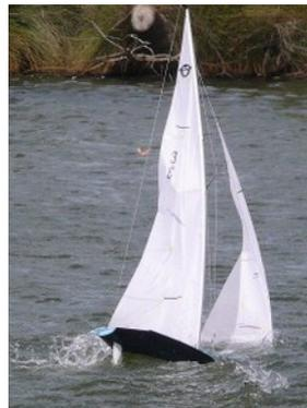
I was recently able to catch a moment during high winds with a boat on the run being driven under water. I was astounded by the amount of mast bend this created (photo left) without the mast breaking. There was certainly the opportunity for breakages.
