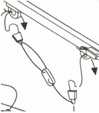
The Seawind building instructions specifies that the sheets are set up (left) using clips to the booms and to cater for adjustment with the supplied bowsies. This works reasonably well with the supplied cord as this does not slip when used with these bowsies.
