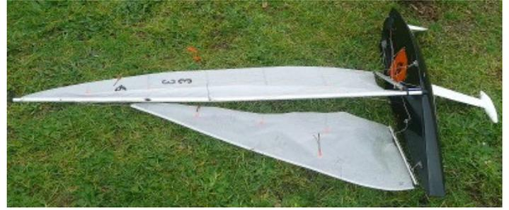
**Wayne:** I managed to panel beat the mast joiner into shape using the vice and a former or two, I worked out it can be flipped upside down and reused to move the weak area away from the joint. I'll go to 75kg cord to prevent the same series of events happening again, twice as strong as the stock cord but a similar diameter.
