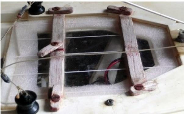
This hatch was made from a broken headlight cover reinforced by a couple of teak strips. Wood blocks were glued under the side decks and teak turning toggles were screwed down. Sheet foam gaskets make this watertight.
