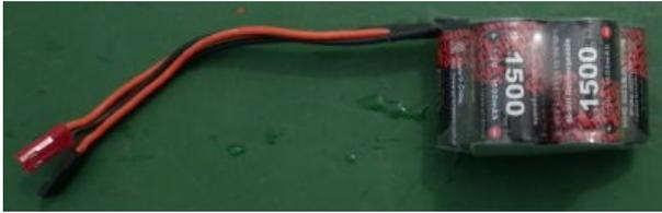
Prebuilt five cell packs are available using short cells so that it will fit in the Seawind holder. These are relatively expensive and would be hard to fix if a cell failed.
