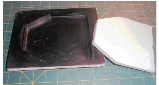
A fibreglass mould is available for members to make their own fibreglass hatch. It produces a tight fitting flush hatch. Sidedeck toggles, or small bolts as above, would be used to hold it in place.
