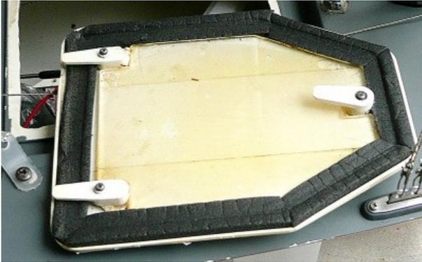
This example has perspex reinforcing cut to fit inside the replacement closed-cell rubber strips.
