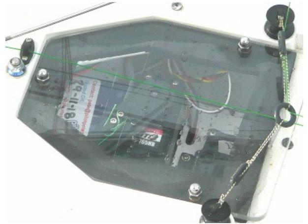
This perspex hatch is held by nuts onto small bolts fixed to the hatchway rim.
