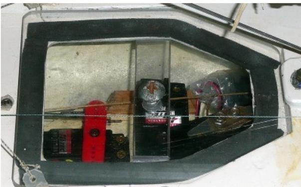
An alternative is to use a bar that turns under the side decks to hold the hatch in place. In this example self-adhesive rubber strips have been attached to the hatch coaming to form a gutter around the strips. The bar is perspex with a captive nut inserted into it. The screw has now been replaced by a stainless steel bolt. A limit stop is glued under the starboard side deck so that the bar only turns to the athwartship position when the bolt is tightened.
