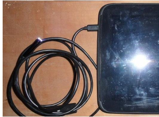
A USB endoscope camera is quite inexpensive and can be attached to a mobile phone or tablet and used to peer inside confined spaces.
