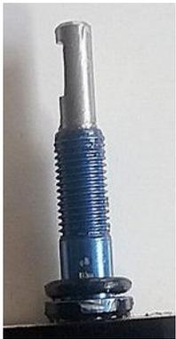
I have found that the tube and rudder have corroded and I cannot free them by using the release agents I have.
