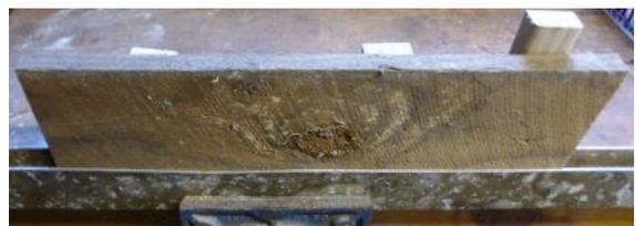
In order to deflect the water from the work area during drilling the half board will be added on top to raise the weir level and a piece of wood can be wedged in to deflect any overspill to be either side.
