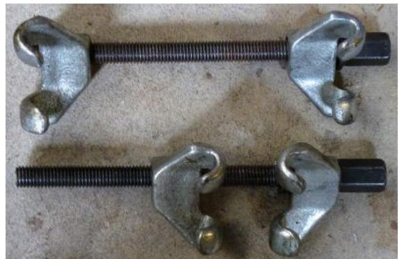
A set of spring compressors has been obtained cheaply at the local market and one (lower) modified to be an expander. It is planned to drill through the top two boards and tread wire through these and make them into loops. The expander can then be used to force these apart.
