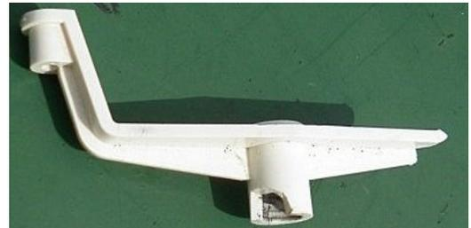
Gary McKenzie was at the pond and showed the cause of his sinking. The rear frame had a section missing around the rudder tube and when the frame side broke it released the pressure and flooded.
