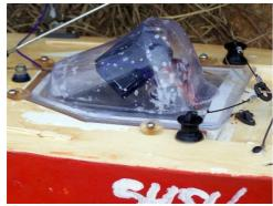
Jim Keogh has equipped his perspex hatch with a bubble cut from some packaging. His 2.4GHz receiver is set up high to keep the aerial above water level and to keep it dry.
