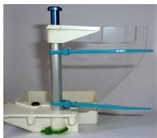
This method of fixing gives two advantages. The support can be installed (with difficulty) without removing the tubes and parts by slipping it into place and tightening the ties. The load is completely removed from part C3 so if this is broken, this can still be installed.
