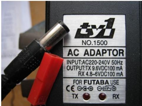
Battery chargers come in many forms. There are special chargers available for radio control that can charge both the transmitter and the receiver batteries at the same time without removing them. The one above is a plug in unit for Futaba radios. It has two output cables: one that plugs into the transmitter and the other takes a battery pack with a standard connector. Note that the output is 100mA (milliAmp) for both voltages.
