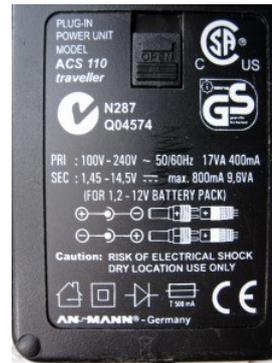
'Smart' chargers are available that will detect the voltage of the pack that is connected to it - this one caters for 1.2 volt to 12 volt packs - and will detect when it has reached full capacity and switch to trickle charging. This model also has a 'discharge' option.
