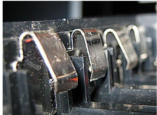
If the transmitter has flat bladed 'springs' then check that these have not been flattened, this can happen if the transmitter is dropped. With less pressure on the battery a bump may jolt the battery to lose contact. 2.4Ghz transmitters can lose connection from a brief power drop, it may take several seconds for it to re-connect to the boat.
