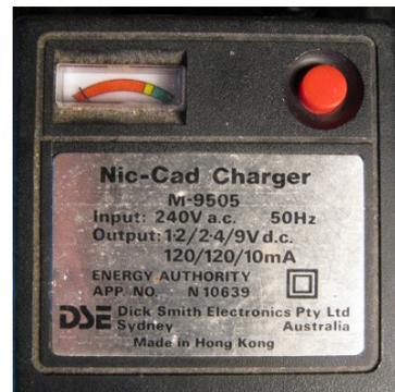
This one has a battery meter in the left hand holder. It outputs 120mA for AA which is sufficient for recharging overnight and is not high enough to damage the cells if left charging continuously.
