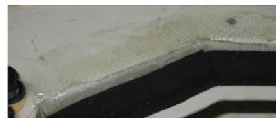
A small piece of fibreglass cloth was added to the outside using epoxy glue.
