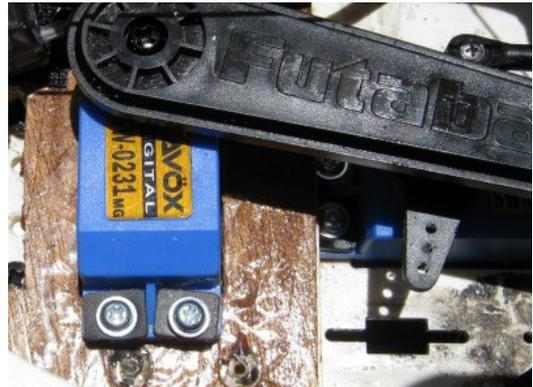
Garry Irwin has rebuilt his old 'Goldie' to replace his other boats. He has installed two AVOX waterproof digital servos. The sail servo is rated at 18 Kg/cm which is greater than the standard HS-765HB. The servo is quite a bit smaller and requires a mounting plate to bridge between the servo screws and the servo tray's post. Garry has made this plate (shown above) of plywood.
