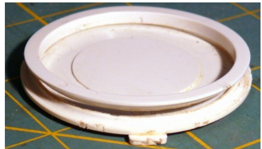
A rear hatch that has split due to 'super glue' failing.
