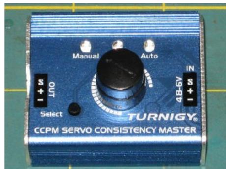
Using special test equipment should give better results. The Turnigy Servo Tester can test and compare up to three servos at a time and has manual and automatic modes, plus a mode to centralise the servo.
